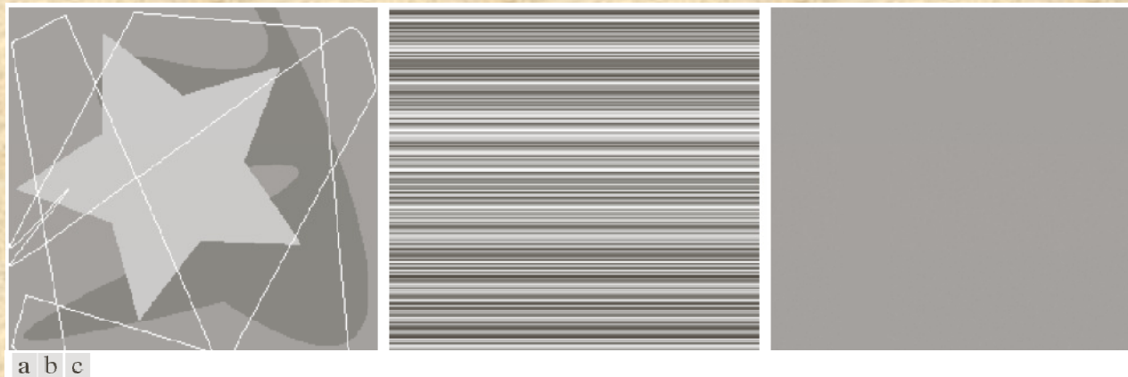
FIGURE 8.1 Computer generated 256 \times 256 \times 8 bit images with (a) coding redundancy, (b) spatial redundancy, and (c) irrelevant information. (Each was designed to demonstrate one principal redundancy but may exhibit others as well.)
