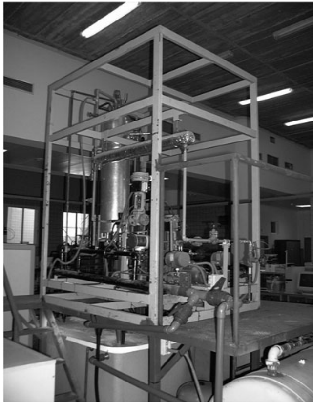
Figure 1. Pilot plant used to apply the proposed nonlinear model predictive control strategy based on the convexification approach.
