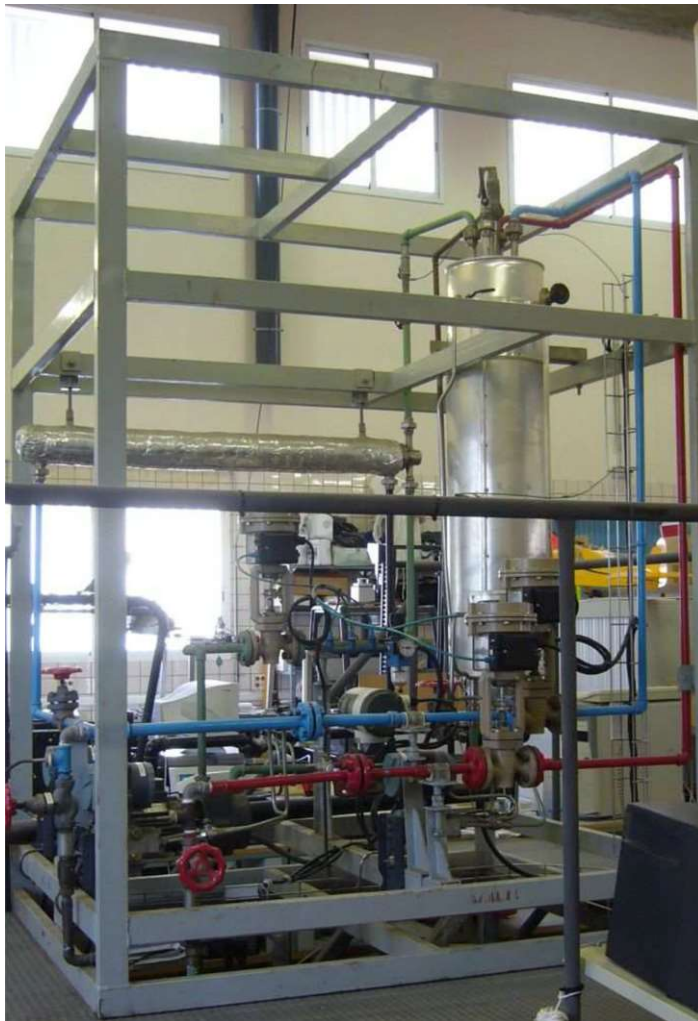
Fig. 2. Pilot plant used to apply the proposed MMMPC based on a Volterra series model.
