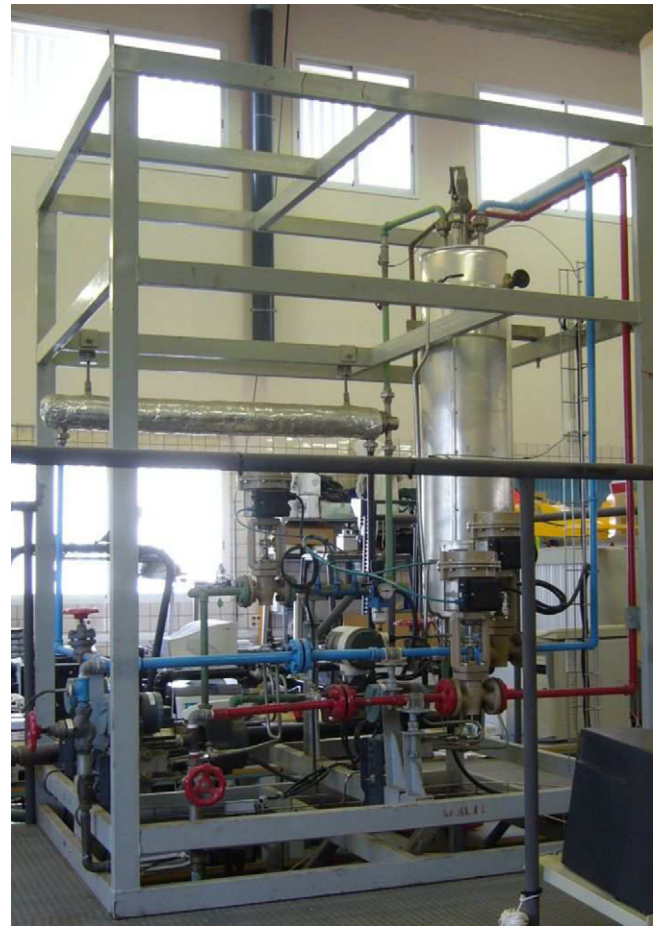
Fig. 2. Continuous stirred tank reactor used to apply the MMMPC based on an upper bound of the worst case cost.
