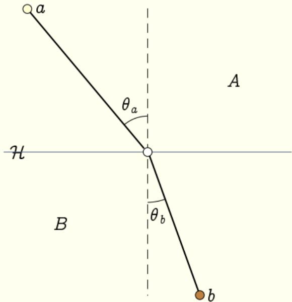
$\omega_A, \omega_B$  refraction indices.
