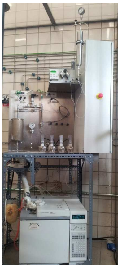
High pressure fixed-bed lab reactor
