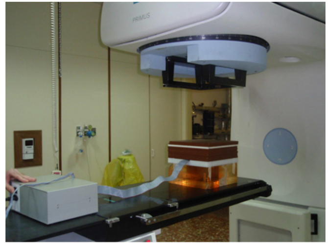
Fig. 1. PRIMUS™ linear accelerator at the Virgen Macarena University Hospital in Seville and the experimental setup with the slab phantom mounted during a test.
